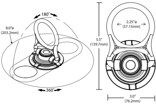
**Tensile Strength (UTS): 5,000-lbf (22kN)**
